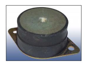
The Flanged Bobbin Mount or DB(L)R range is composed of a rubber block bonded to an upper threaded plate and a lower metal flange. The flanged bobbin mountings are the generating set industry standard non-fail safe mountings. These bobbin mounts are easily fitted to engines, alternators, floors and chassis. Flanged Bobbin Mountings have been designed for providing low shear stiffness rates with large compression stiffness rates.
