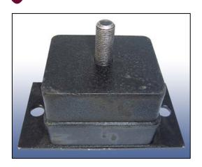
Engine mountings allow for high vertical static and shock loads in compression, whilst simultaneously providing for high isolation values in horizontal shear.
